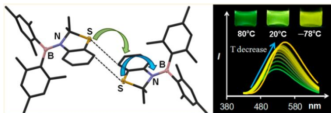
Figure 1. The proposed mechanism of excimer emission and its shift with decreasing temperature
